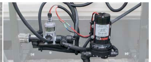
Electric pump and boom control
