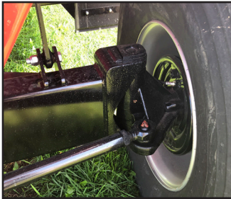
Cast Spindle Carriers - front and rear
