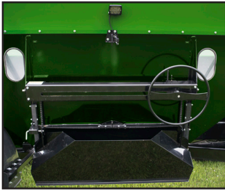
Adjustable Door Opener with Larger Hand Wheel
