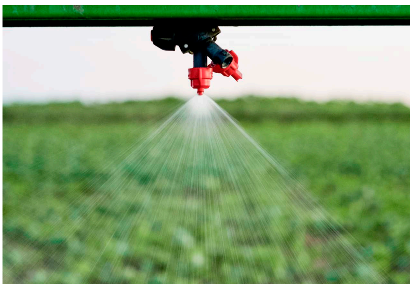
SoftDrop SD110-04 nozzles field testing in Germany
