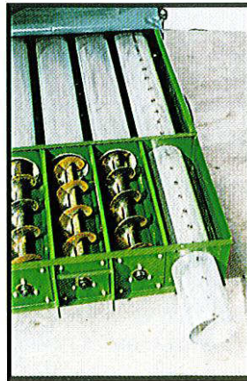
Hopper & End Plate Removed to Change Screens
