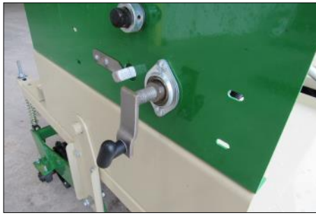
Simple & Highly Accurate Fluted Seedcup Adjustment System
