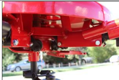
Spheroidal cast iron cam and steel rollers.
