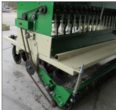
High Precision Ground Drive Seeding System.
