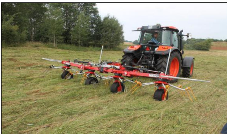
Thick-Walled Tubular Tine Arms
