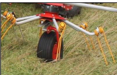
Thick-Walled Tubular Tine Arms
