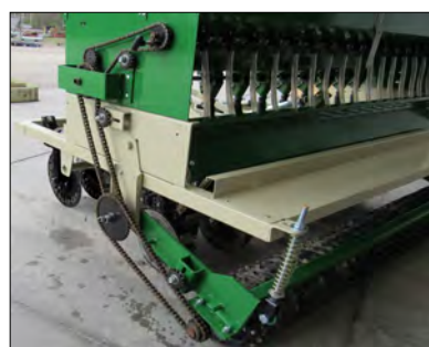
High Precision Ground Drive Seeding System.
