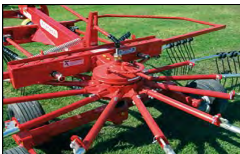
Heavy Duty, Sealed Oil Bath G-box
