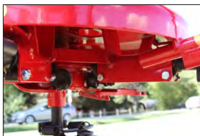
Spheroidal cast iron cam and steel rollers.
