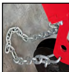
Heavy chain to ensure seed coverage
