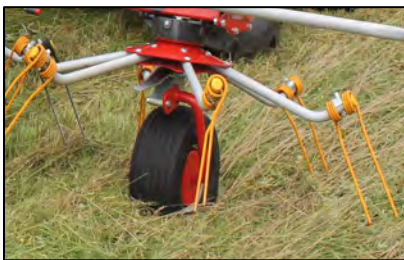
Thick-Walled Tubular Tine Arms
