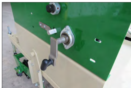
Simple & Highly Accurate Fluted Seedcup Adjustment System
